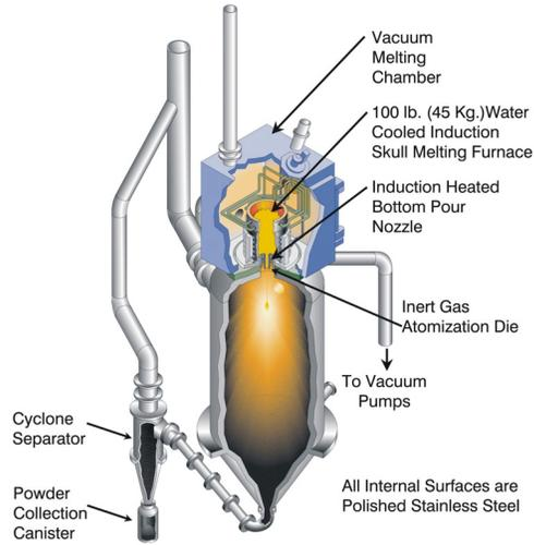
Figure 1. Titanium gas atomization system. (100lb)
