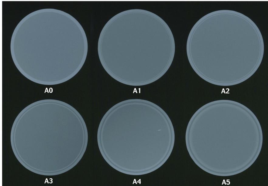
Figure 12. Radiographs of 395MM 3mm thick disks HIPed at the temperatures indicated in Table VI.
