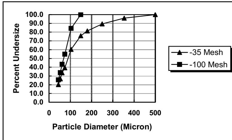
Figure 4. Size distribution of gas atomized gamma titanium aluminide powder.
