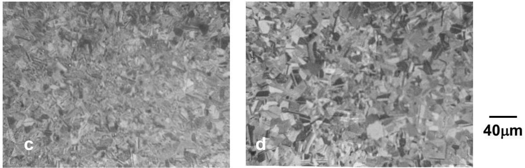
Figure 7. As-HIP microstructures of 318mm diameter by 813mm 395MM compact in different locations in compact a.) top, edge b.) top, center c.) bottom, edge d.) bottom, center
