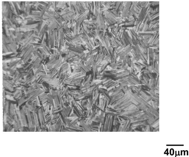
Figure 8. Fully lamellar microstructure in HIP plus heat treated (1360C) 395MM
