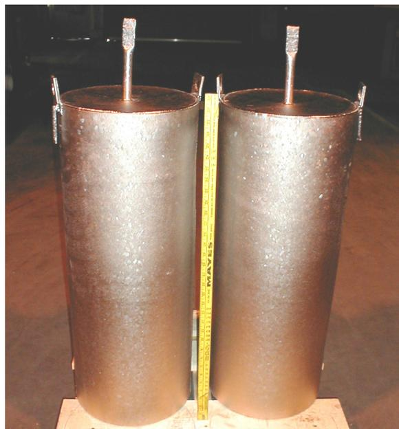
Figure 5. As-HIP 318mm (12.5 in.) diameter by 813mm (32.0 in) 395MM compacts
