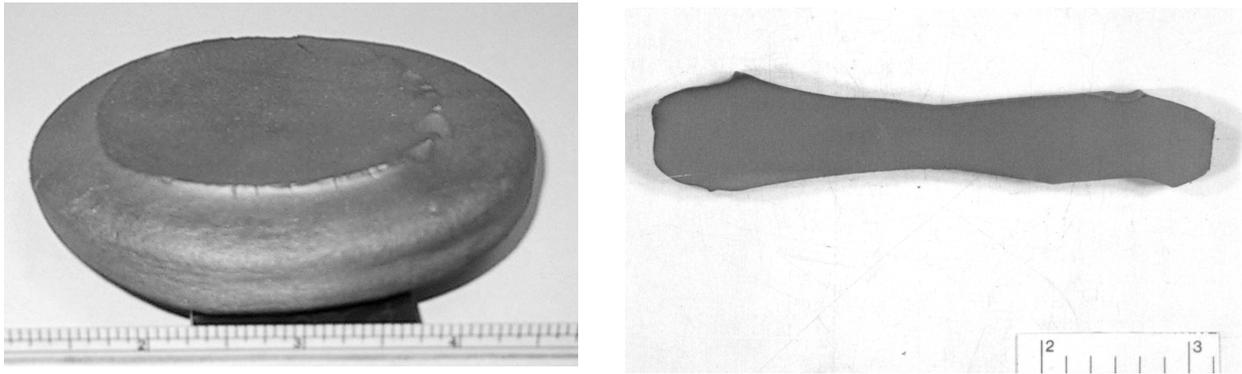
Figure 9. As-forged 395MM pancake and cross-section.
