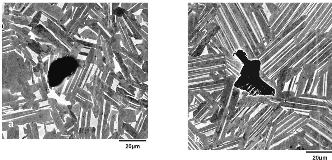
Figure 14. Pores in HIPed plus heat treated disks a) HIPed at 1200C and heat treated for 2h at 1360C b) HIPed at 1400C and heat treated for 2h at 1360C
