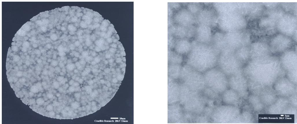
Figure 3. Cross-section of as-atomized Ti-47Al- 2Nb-2Cr (at%) powder.
