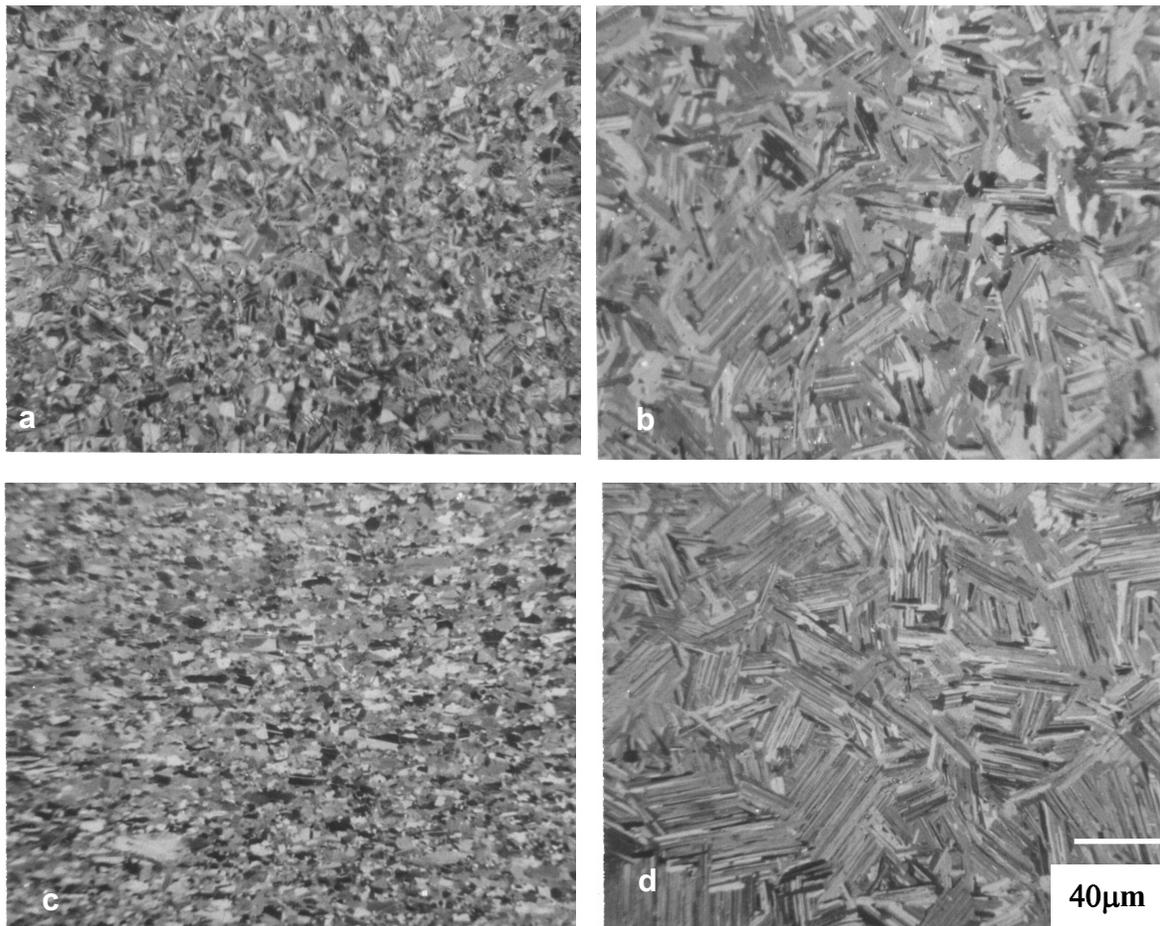
Figure 10. Microstructures of HIPed and forged 395MM compact. a.) As-HIP 1260C (2300F) b.) HIP + 1370C (2500F) 1h AC + 950C (1740F) 8h c.) As-forged 1260C (2300F) d.) Forge + 1370C (2500F) 1h AC + 950C (1740F) 8h
