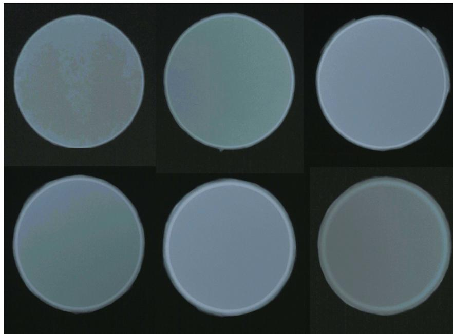
Figure 13. Radiographs of 395MM 3mm thick disks HIPed and heat treated at 1360C (2480F) for 2h.
