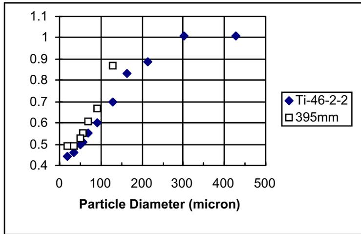
Figure 11. Argon content of gas atomized titanium aluminide powder vs particle size.
