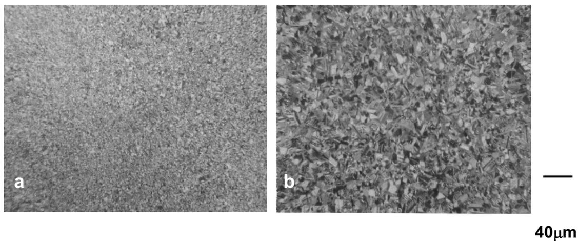
Figure 6. As-HIP microstructures of 395MM alloy. (a) HIP 1000C, (b) HIP 1280C.
