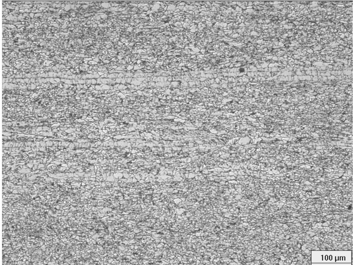
**Fig. 10 Optical micrograph of mixed grains**
