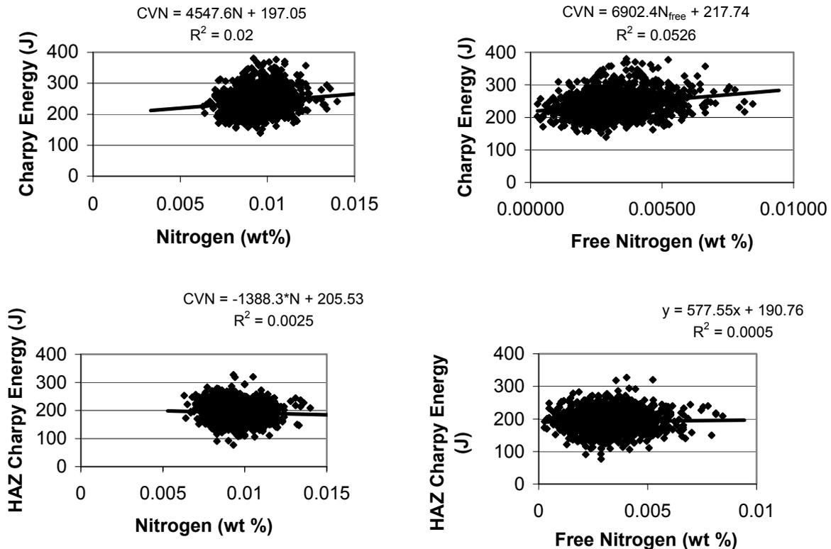
Figure 9. Effect of nitrogen on Charpy energy at  $-7^{\circ}\text{C}$ .
