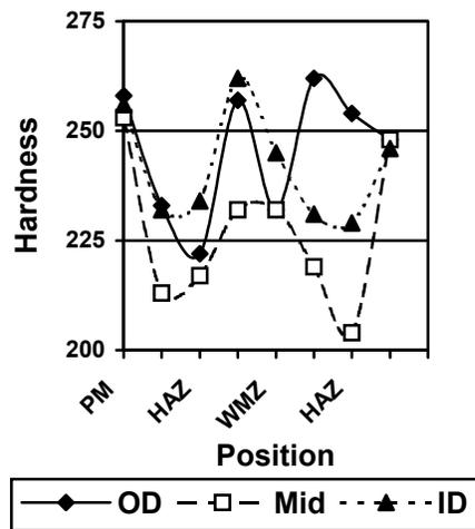
Figure 7. Hardness profile of spiral weld on 0.667 ins. pipe.
