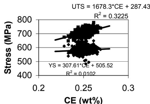
Figure 10. Effect of carbon equivalent (CE) on YS and UTS.
