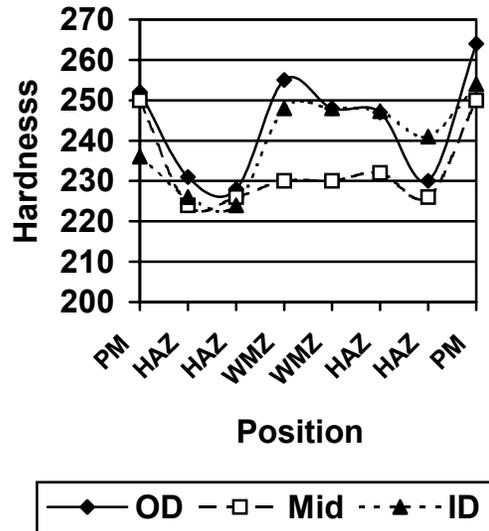
Figure 5. Cross section of Spiral weld and corresponding hardness profile.
