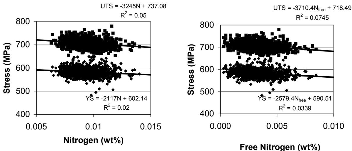
Figure 8. Effect of nitrogen and “free” nitrogen on tensile properties.
