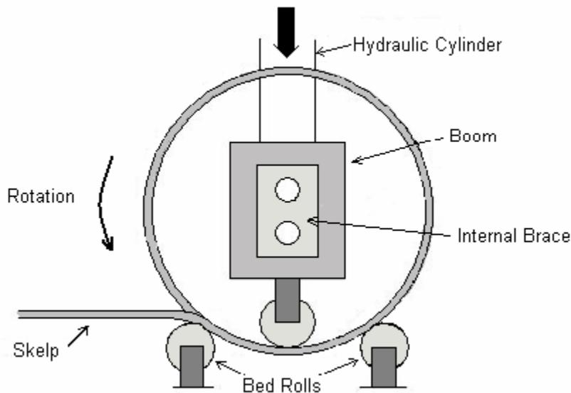
Figure 4. Schematic of the boom and bed rolls.
