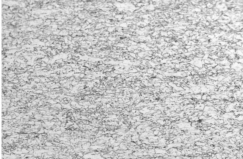
Figure 2. Microstructure of as-rolled skelp.
