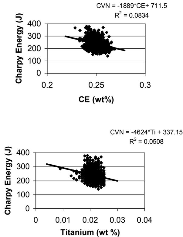
Figure 12. Effect of carbon equivalent ( $CE_{CSA}$ ) and Ti on Charpy energy at  $-7^{\circ}C$ .
