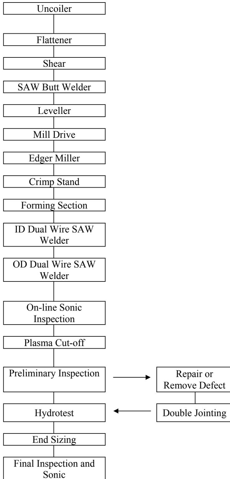
Figure 3. Spiral Mill Operations Flow Chart.
