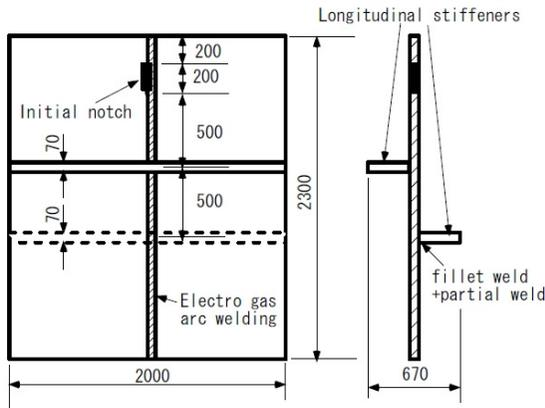
Figure 5. Dimensions of specimen [6].
