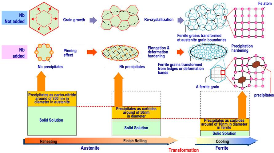
Figure 1. Niobium precipitation at each stage of TMCP and its effects on refining of ferrite grains and precipitation hardening [1].
