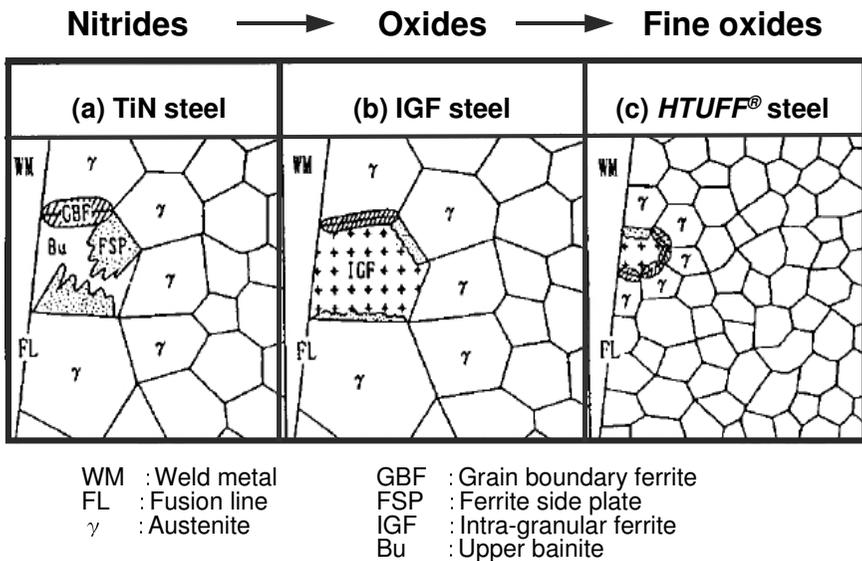
Figure 12. Examples of development in technology for improving HAZ toughness [16].
