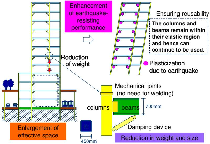
Figure 11. New construction system using high-strength steels [10].
