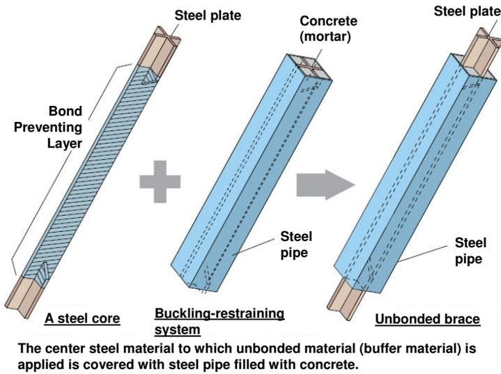
Figure 10. Structure of unbonded brace [14].
