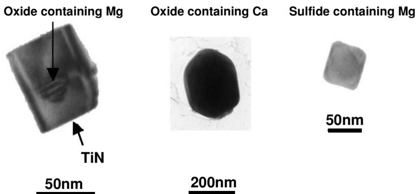
Figure 13. Examples of pinning particles of HTUFF® steel [16].
