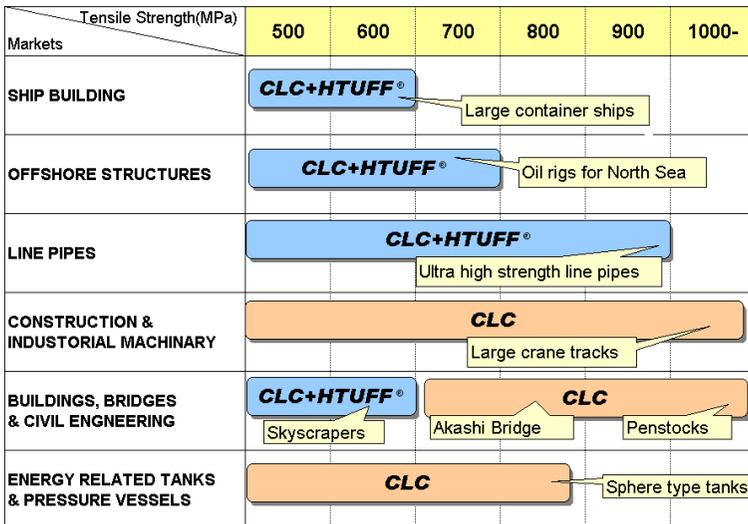
Figure 2. Strength level of TMCP and HTUFF® steel plates for each market.
