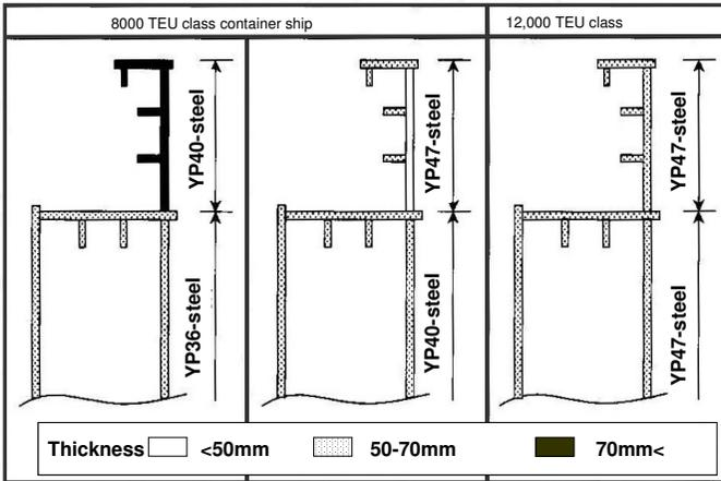
Figure 8. Examples of hull structures in mega-container ships [4].
