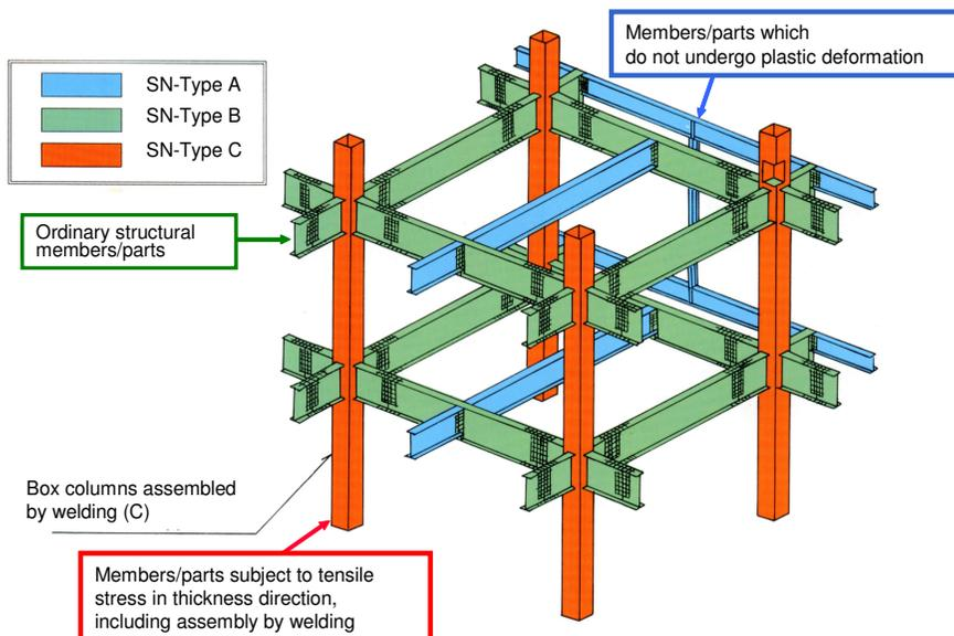
Figure 9. Points of application of SN steel [10].
