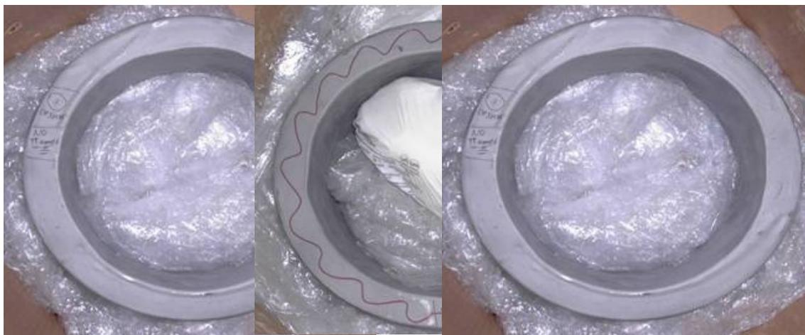
Figure 1. Cast Allvac 718Plus rings produced at PCB.
