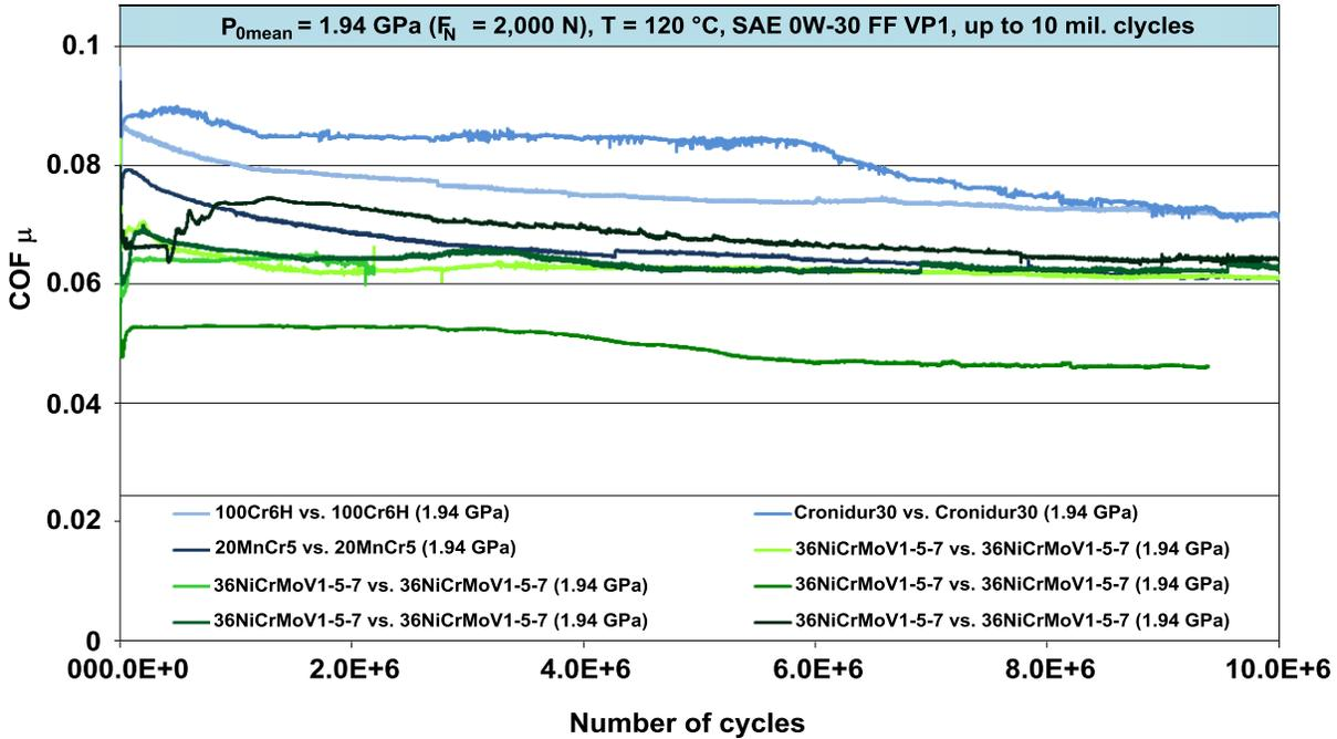
Figure 12. Evolution of the coefficient of friction over the test period of 10 million load cycles at  $P_{0\text{mean}} = 1.94 \text{ GPa}$  and  $T = 120 \text{ }^\circ\text{C}$  in SAE 0W-30 VP1 oil.
