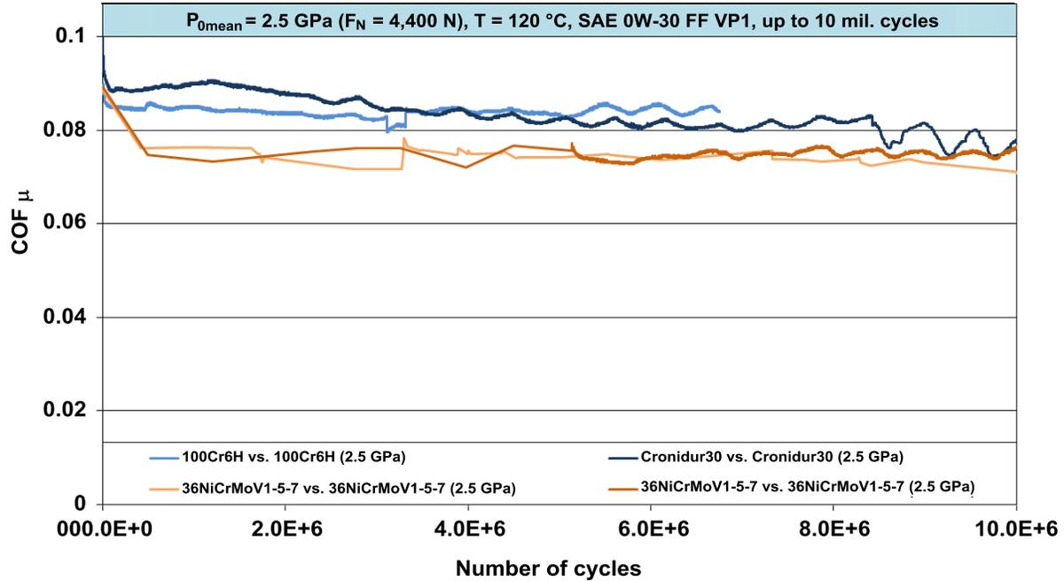
Figure 13. Evolution of the coefficient of friction over the test period of 10 million load cycles at  $P_{0\text{mean}} = 2.5 \text{ GPa}$  and  $T = 120 \text{ }^\circ\text{C}$  in SAE 0W-30 VP1 oil.
