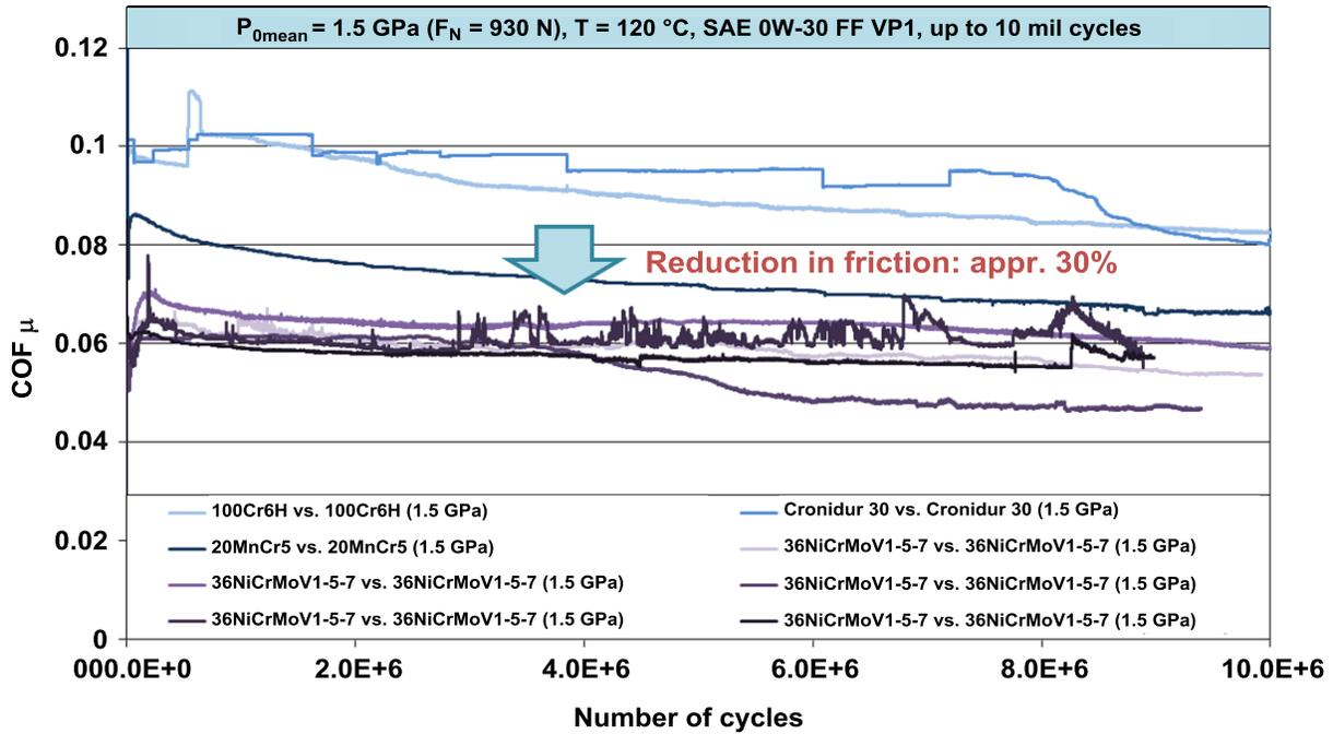
Figure 11. Evolution of the coefficient of friction over the test period of 10 million load cycles at  $P_{0\text{mean}} = 1.5 \text{ GPa}$  and  $T = 120 \text{ °C}$  in SAE 0W-30 VP1 oil.
