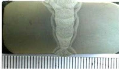
Figure 11. GMAW welded joint macrograph.
