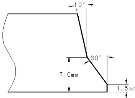
Figure 14. GMAW + FCAW Process Bevel.
