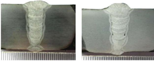
**a) root incomplete penetration    b) lack of fusion between layers**
