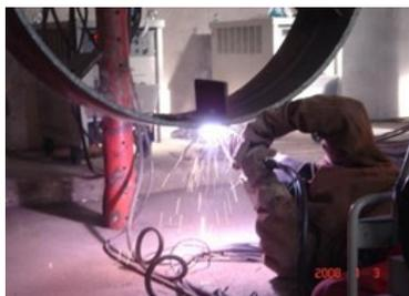
Figure 4. Self-shielded flux-cored wire semi-automatic welding PQR.
