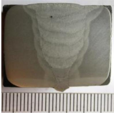
Figure 15. GMAW + FCAW welded joint macrograph.
