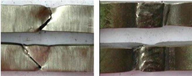
Figure 6. Welded joint tensile fractures in the HAZ area.
