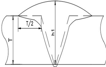
Figure 7. Geometric reinforcement weld design
