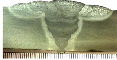
Figure 8. Geometric reinforcement example
