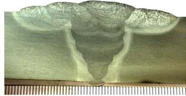
Figure 8. Geometric reinforcement example
