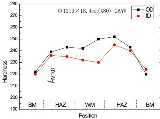
Figure 12. GMAW hardness testing.
