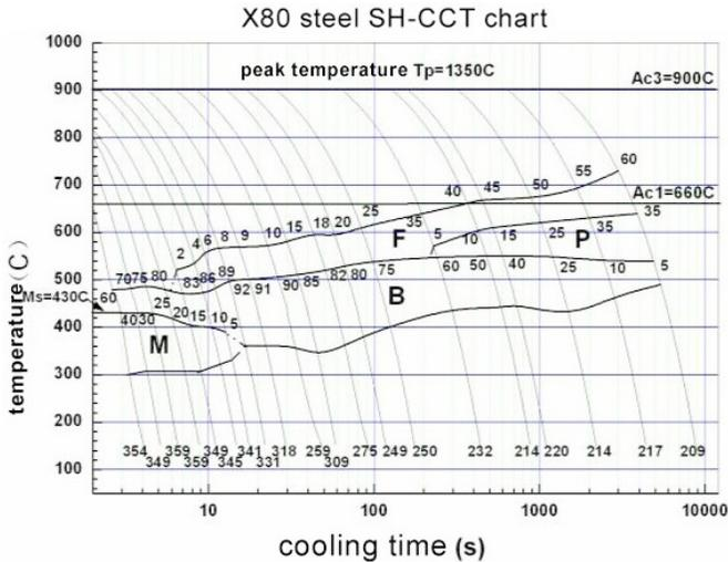
Figure 5. X80 line pipe SH-CCT chart for the Second West–East Pipeline Project.
