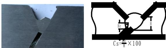
Figure 2. Cross-section of oblique Y-groove welded seam.
