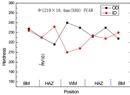
Figure 16. Hardness test results.
