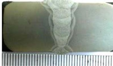
Figure 11. GMAW welded joint macrograph.
