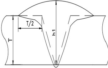
Figure 7. Geometric reinforcement weld design
