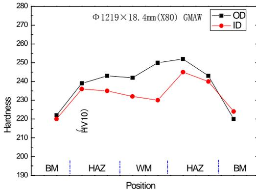
Figure 12. GMAW hardness testing.
