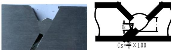
Figure 2. Cross-section of oblique Y-groove welded seam.
