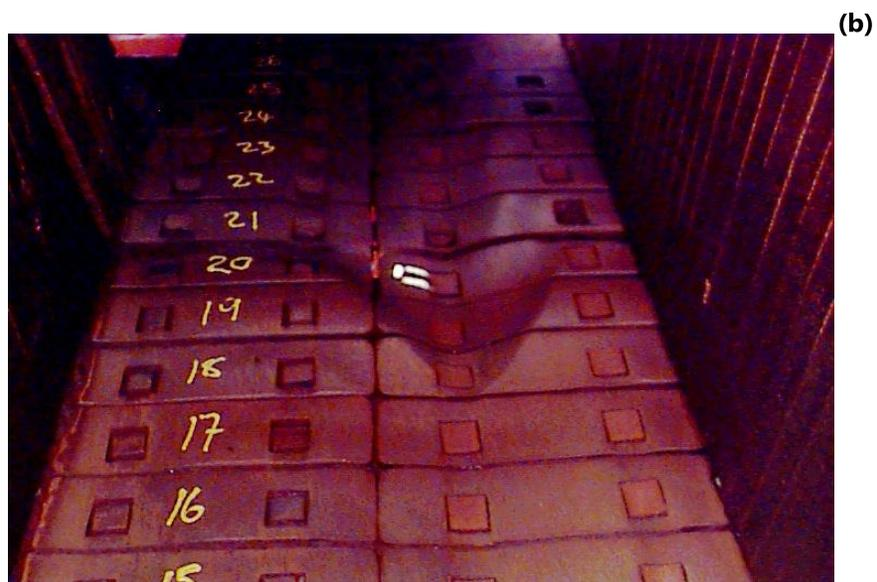
Figure 9. Cast liner blocks in the lower “spoon” section of the live chute; photographs taken at different times in 2000. Wear intensity varies strongly both longitudinally and laterally. Moreover, the point of maximum wear was seen to shift from week to week — compare location of high-wear zone in (a) with that in (b). In addition to intense wear at the freefall impingement point, preferential wear can also be discerned below (downstream from) the open bolt recesses.
