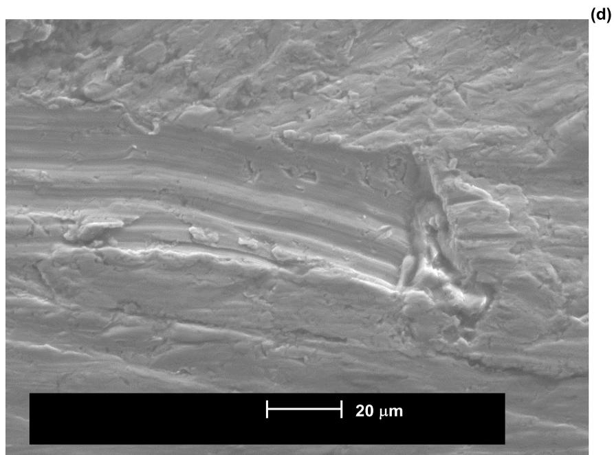
Figure 20. SEM secondary electron images comparing the worn surface characteristics from the pug mill trial with those from the IC-SBAT with the same greywacke abrasive; (a) Pug mill worn surface at low-medium magnification, (b) IC-SBAT worn surface at low-medium magnification, (c) Pug mill at medium-high magnification, (d) IC-SBAT at medium-high magnification.
