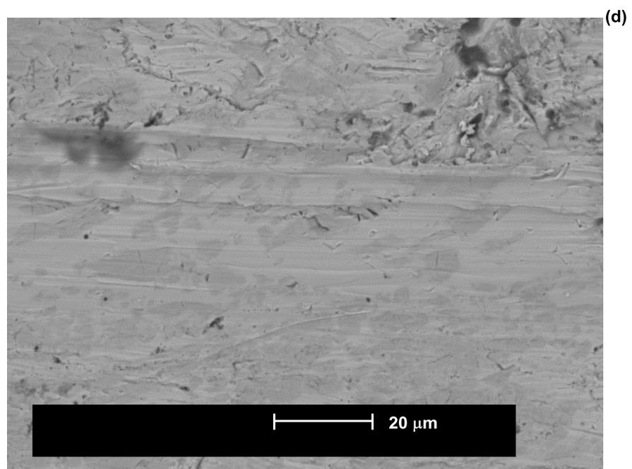
Figure 21. SEM backscattered electron images; (a), (b) Pug mill and IC-SBAT worn surfaces at medium-high magnification, (c), (d) Pug mill and IC-SBAT worn surfaces at high magnification.
