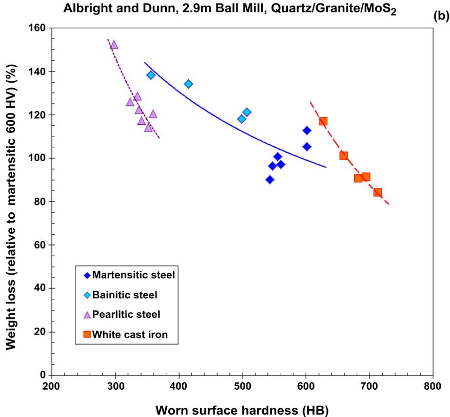
Figure 1. Re-plot of data extracted from Albright and Dunn 1983 [3] (similar to those presented in Figure 2 of Gates et al. 2007 [4]). After identifying the four alloy classes, wear rate relative to martensitic steel of hardness 600 HV is plotted against worn surface hardness.
