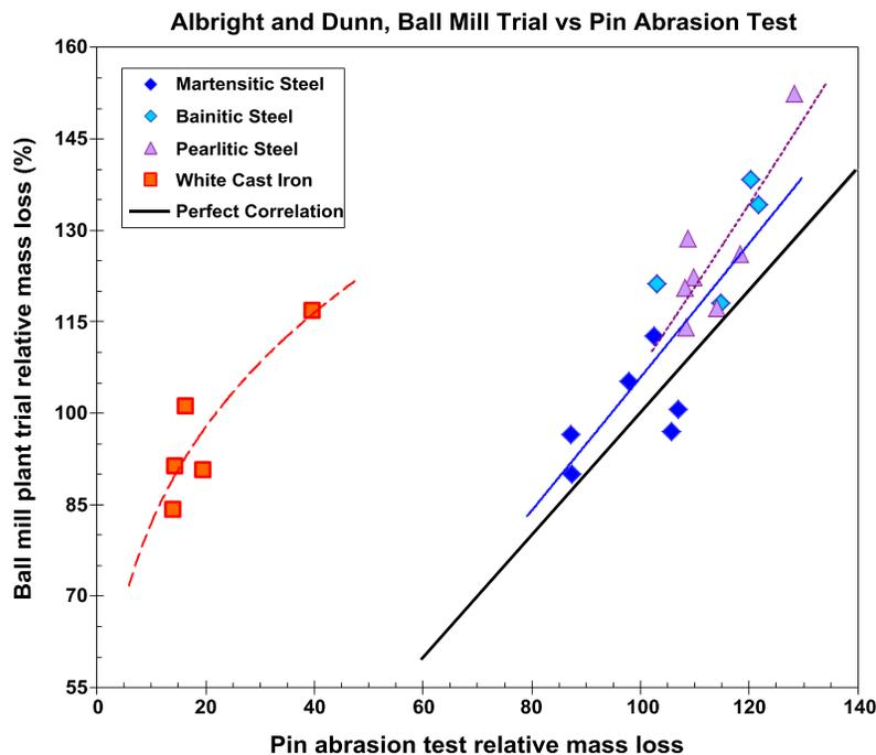
Figure 2. Re-plot of data extracted from Albright and Dunn [3]. Directly compares wear rates from the industrial ball mill trial (grinding quartz and granite) against those for the same alloys in the pin abrasion test (using 150-mesh garnet cloth).
