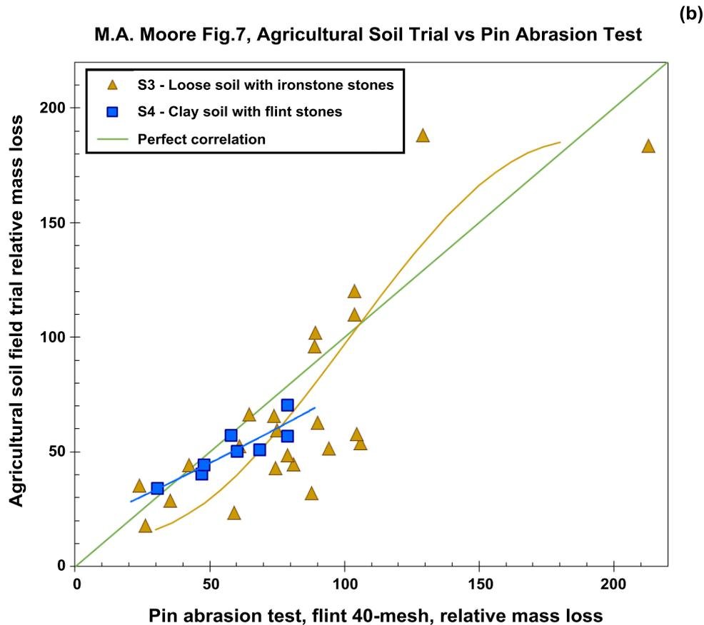
Figure 3. Re-plotted data from Moore 1987 [1] directly comparing wear rates from agricultural field trials against those for the same alloys in the pin abrasion test; (a) using 180-mesh flint, (b) using 40-mesh flint.
