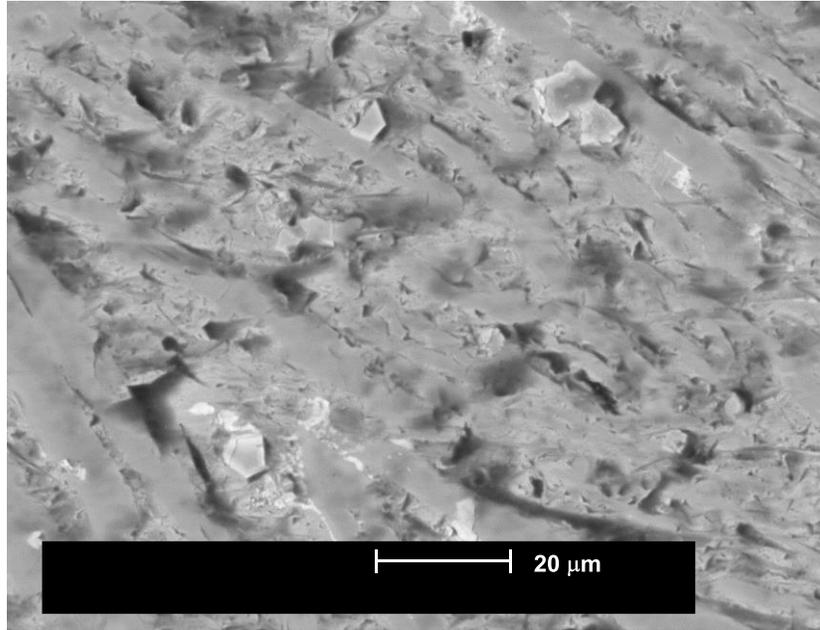
Figure 22. SEM images showing the worn surface of the NbVTi-bearing alloy F in the IC-SBAT with greywacke. The Nb-rich carbides stand proud of the matrix, and evidently provide a measure of protection to the host alloy despite their low volume fraction.
