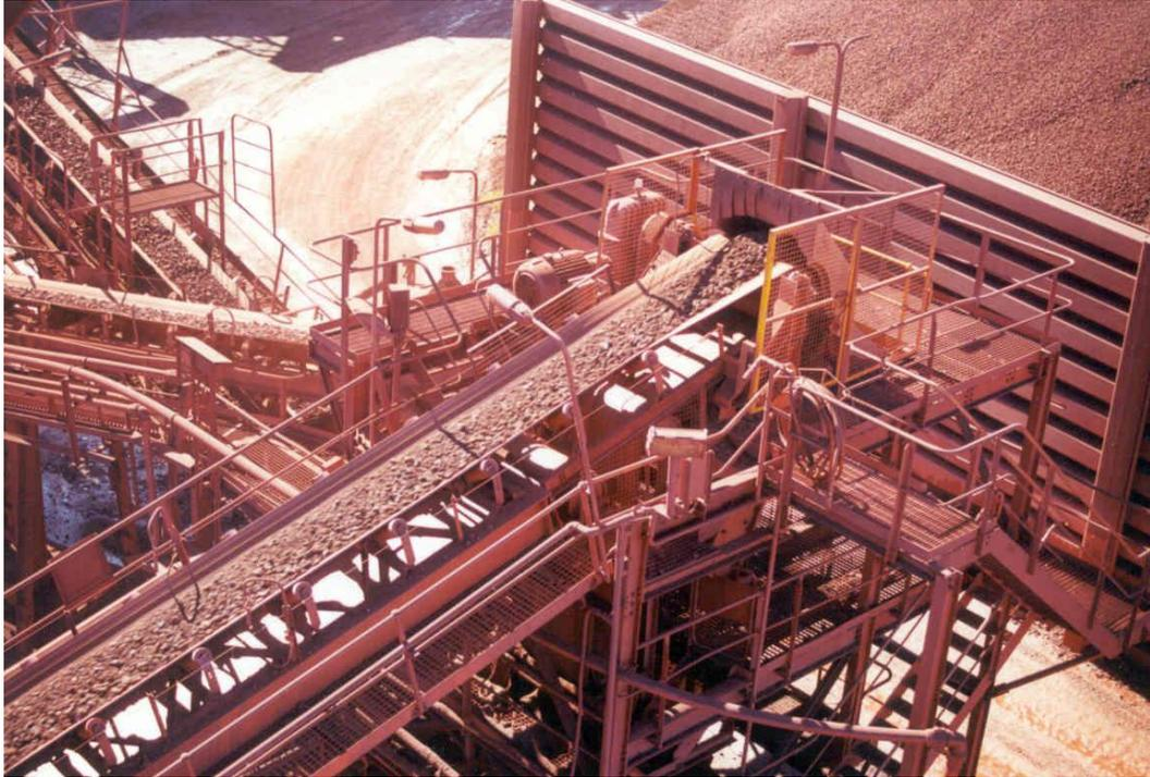
Figure 7. CN40/CN42 transfer station at BHP Iron Ore's Finucane Island operation in 2000, with Tasman Warajay "Controlled Flow" chute.
