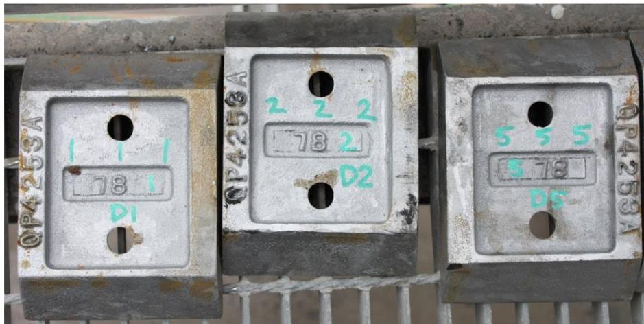
Figure 17. Paddles ready for installation in the pug mill trial. Paddles A were the OEM paddles, B the after-market paddles, D and F were alloys cast for the purposes of the trial.
