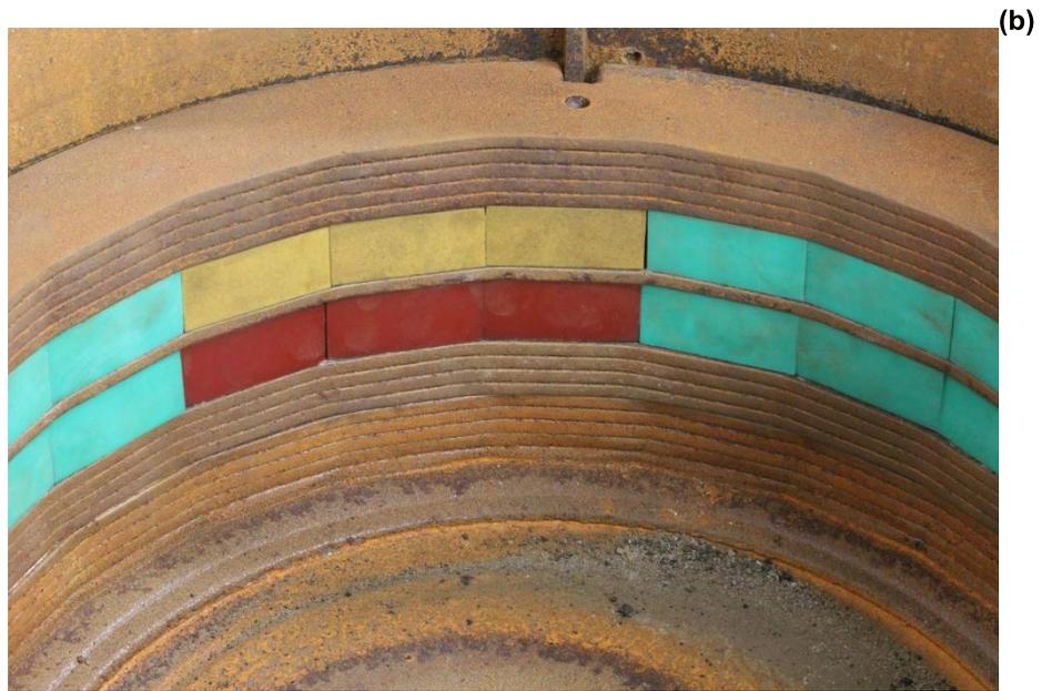
Figure 13. Different specimen sets installed in the IC-SBAT; (a) Mild steel specimens used for commissioning trials, (b) Polymeric wear-resistant materials, including polyurethanes and ultra-high molecular weight polyethylene, installed for a consultancy project.
