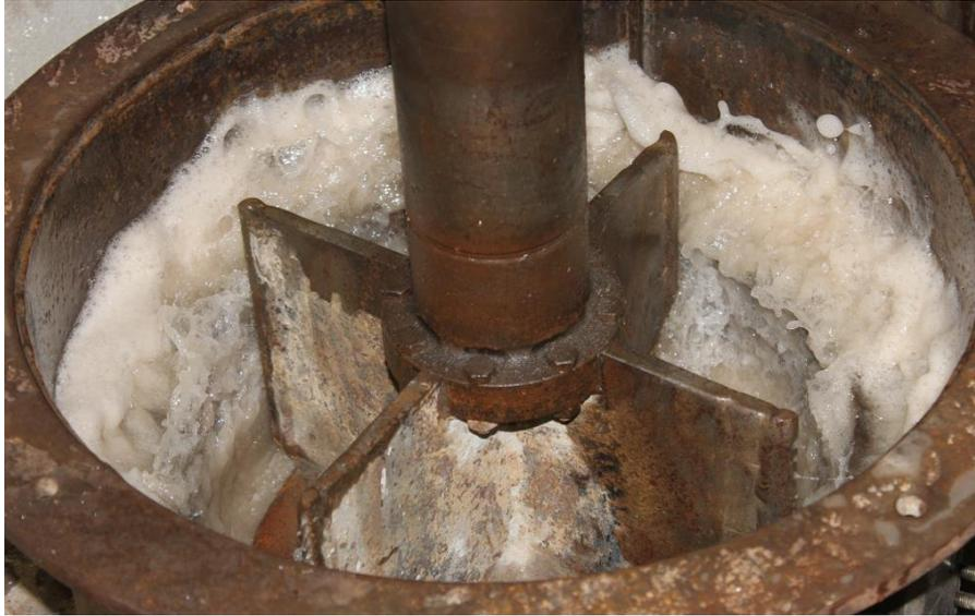
Figure 14. Operation of the IC-SBAT device in wet particle erosion mode (IC-WPET).
