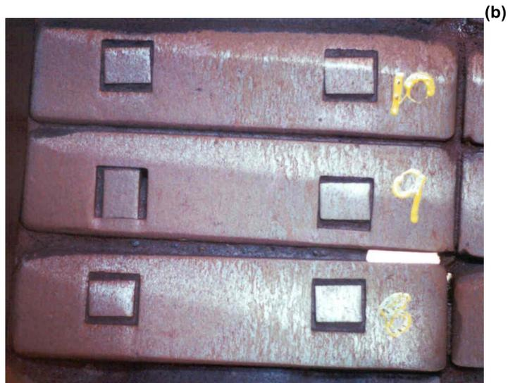
Figure 11. The lower “spoon” section of the live chute at Port Hedland. Shows the damaging effect of open bolt recesses ((a), black solid-headed arrows), the modest improvement obtained from hardened 4140 steel bolt caps ((a), red open-headed arrows), and the greater improvement obtained by use of white cast iron bolt caps (b).
