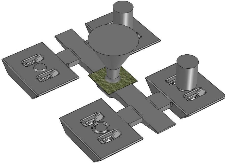
Figure 16. CAD model for the paddle castings that were manufactured in various white cast iron alloys for purposes of the pug mill trial.
