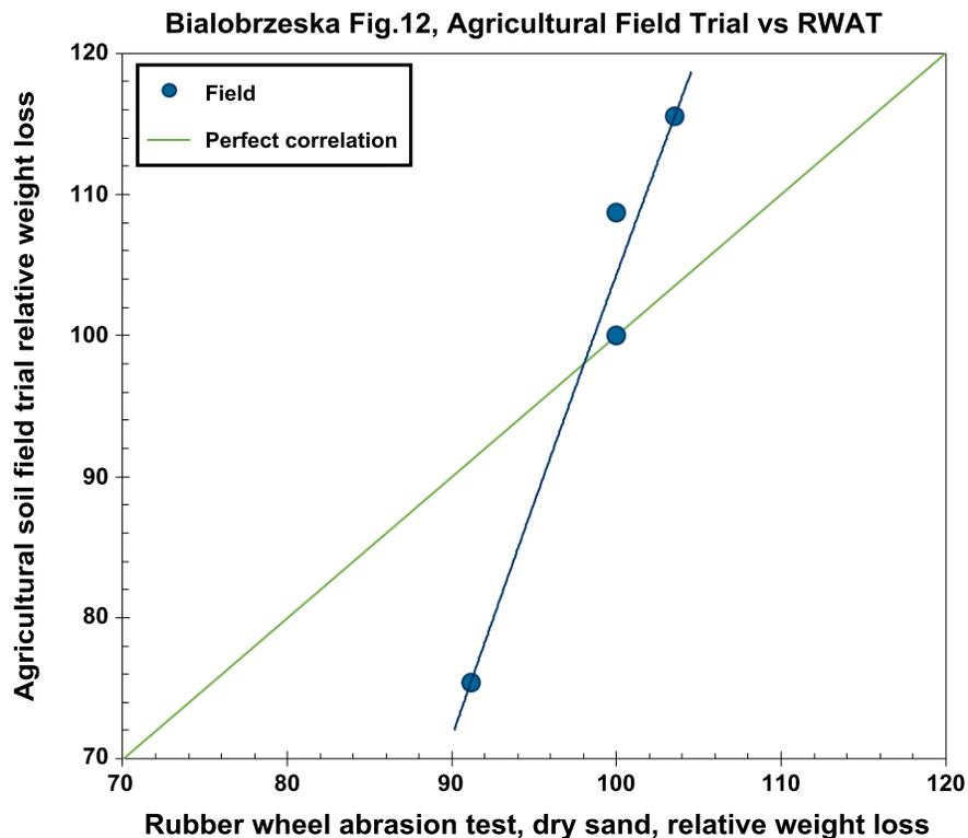
Figure 4. Re-plotted data from Bialobrzaska and Kostencki 2015 [9], directly comparing wear rates from an agricultural field trial against those for the same alloys in the rubber wheel abrasion test.
