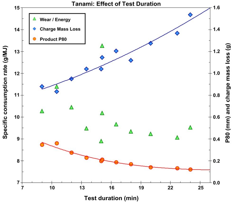
Figure 5. Effect of test duration on 80% passing size of product (secondary axis), charge mass loss (secondary axis), and specific consumption rate (primary axis).
