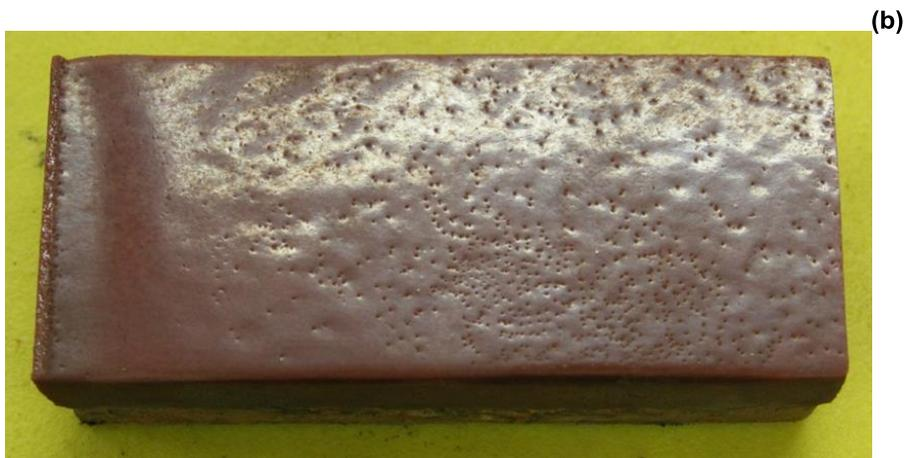
Figure 15. Worn specimens after testing in the IC-SBAT device when operated in wet particle erosion mode (IC-WPET); (a) Stippled surface of mild steel specimen, due to erosion-corrosion (scale millimetres), (b) Polyurethane specimen showing impingement zone behind the leading edge (specimen 55×25 mm, particle flow from left to right).
