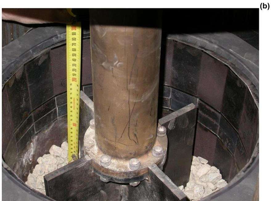
Figure 12. Key design features of the IC-SBAT (inner-circumference sliding bed abrasion test);
