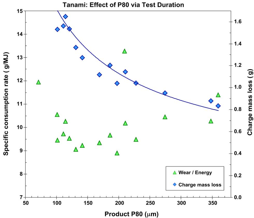
Figure 6. Effect of P80 (varied via test duration) on charge mass loss (secondary axis) and specific consumption rate (primary axis).
