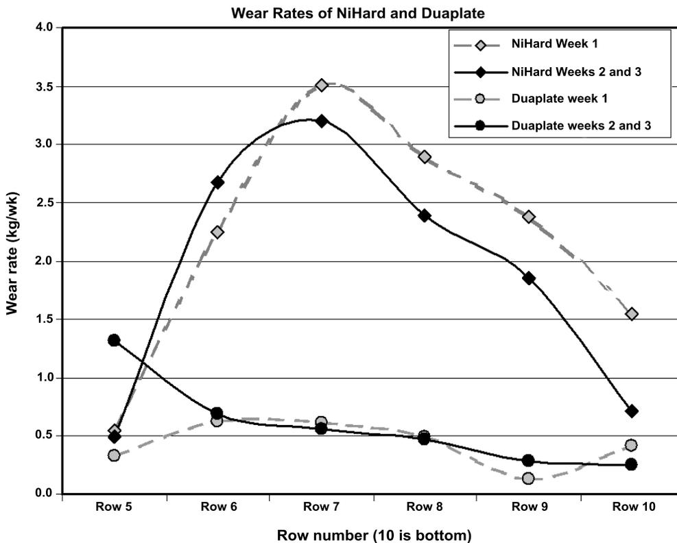
Figure 10. Wear rate measurements from plant trial in hood section of live chute passing iron ore at 1,800 tonnes per hour. Trial used planar array design with plate segments in two alloy products - cast NiHard 4 and Duaplate weld overlay.
