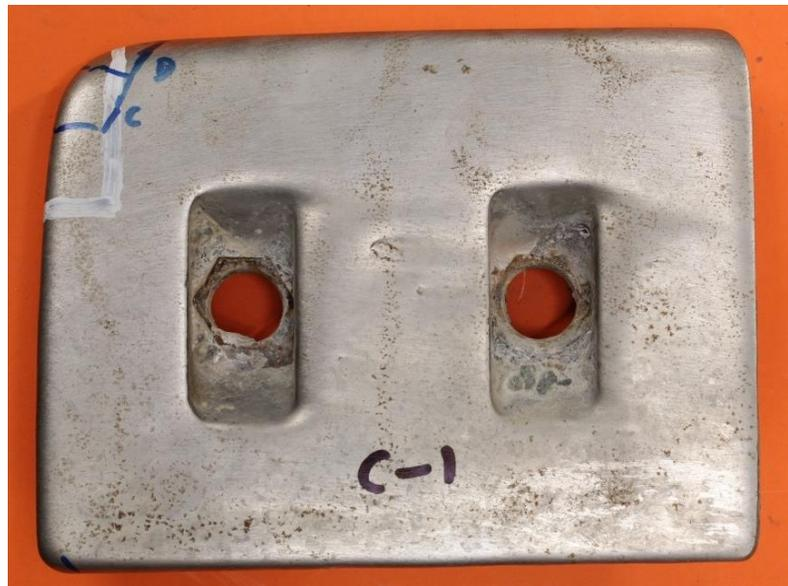
Figure 19. Worn paddles recovered after the pug mill trial, marked for cutting of samples for SEM examination of worn surfaces.
