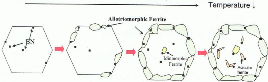
Figure 11. Schematic illustration of the mechanism of boron affecting the phase transformation of the coarse grain region of HAZ.
