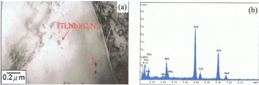
Figure 3. (a) TEM photograph showing the (Ti,Nb)(C,N) particles on the prior austenite grain boundary of the Ti-B treated steel, (b) EDAX analysis pattern.
