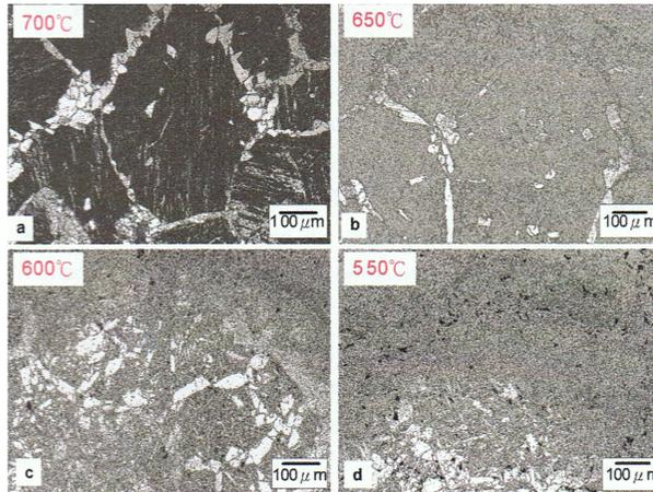
Figure 10. Optical micrographs obtained from four simulated HAZ thermal cycles interrupted at various temperatures: (a) 700°C, (b) 650°C, (c) 600°C and (d) 550°C.
