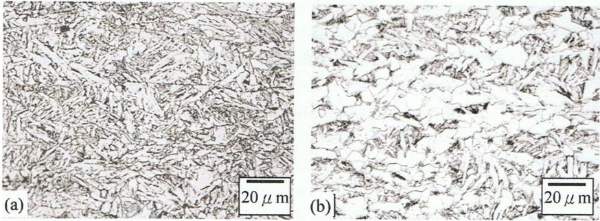
Figure 2. Optical micrographs showing the microstructures of the as-rolled steels: (a) Ti-B treated and (b) B-free.
