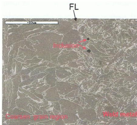
Figure 8. Scanning electron micrograph of coarse-grain microstructure in HAZ of Ti-B steel.
