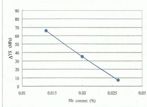
Figure 4. Effect of Nb on the drop of YS (anti-softening behaviour) of EH40 steel plate subject to 400 kJ/cm high heat input welding.
