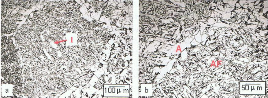
Figure 7. (a) The coarse-grain microstructure in the HAZ of Ti-B treated steel welded by 400 kJ/cm heat input, 9b0 high magnification of (a), (A: Allotrimorphic ferrite, AF: Acicular ferrite and I: Idiomorphic ferrite).
