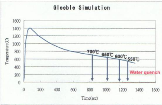
Figure 1. Schematic illustration of the thermal cycle of simulated HAZ.
