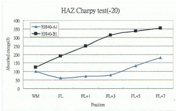
Figure 5. Charpy impact energy versus notch locations of the 400 kJ/cm HHIW HAZ specimens (T-direction). (B1: Ti-B treated, A1: B-free)
