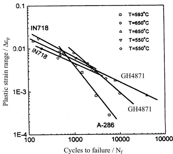
Fig.4 A comparison of LCF properties of GH4871 (AIM+ESR) with A-286 and IN718 alloys
