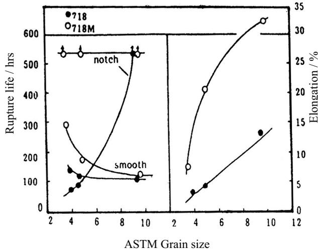
Fig.8 Mg and grain size effect on stress rupture life and elongation at 650°C, 686MPa
