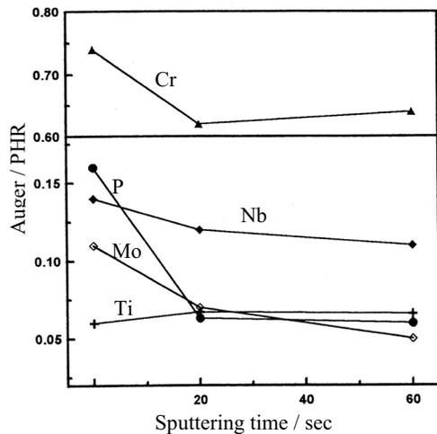
Fig.13 The concentration of P and various elements as a function of ion sputtering time from intergranular fracture surface of IN718 at auger analyses
