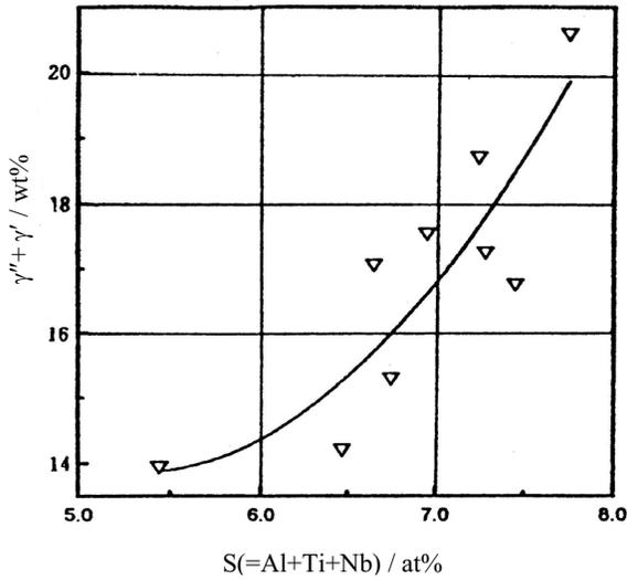
Fig.15 Relationship of (Nb+Ti+Al)% and  $\gamma''+\gamma'$  in modified 718 alloys
