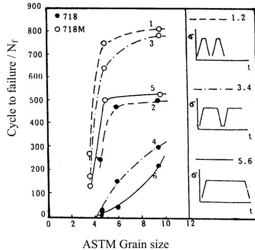
Fig.9 Mg and grain size effect on cyclic stress rupture life with different holding times at maximum stress of 686MPa, 650°C
