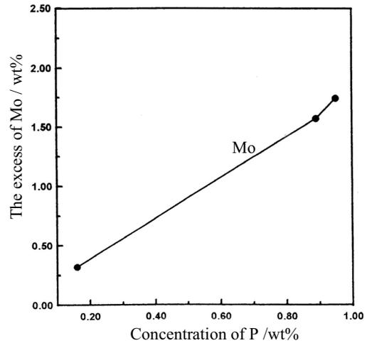
Fig.14 The relationship of Mo and P concentration at grain boundaries (in average)
