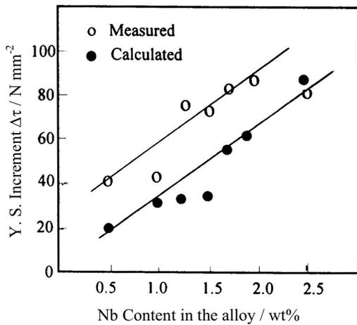
Fig.21 The effect of Nb on yield strength (Y. S.) increment
