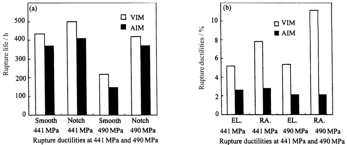
Fig.3 A comparison of 650°C stress rupture properties of air melted (AIM+ESR) and vacuum melted (VIM+ESR) GH4871 alloys
