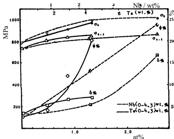
Fig.23 The influence of Ta and Nb in alloys on tensile properties at 760°C
