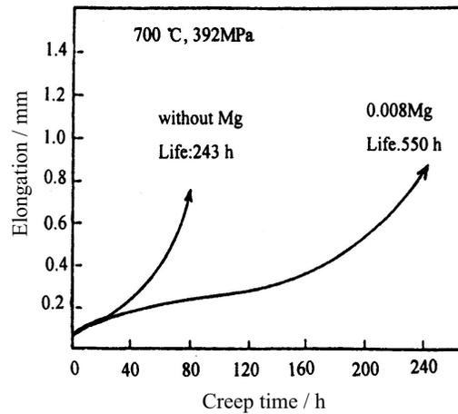
Fig.22 The effect of Mg on creep curves of GH4133
