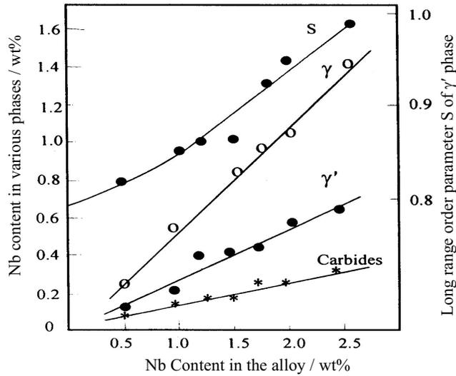
Fig.20 The distribution of Nb in  $\gamma$ ,  $\gamma'$  and carbides and the effect of Nb on long range order parameters of  $\gamma'$  phase
