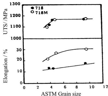
Fig.7 Mg and grain size effect on 650°C tensile properties of Inconel 718
