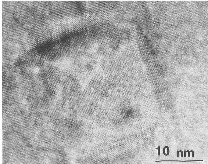
Fig.17 HREM image of compact morphology of  $\gamma''$  and  $\gamma'$  in Alloy 15 after long-time aging at 730°C for 200hrs
