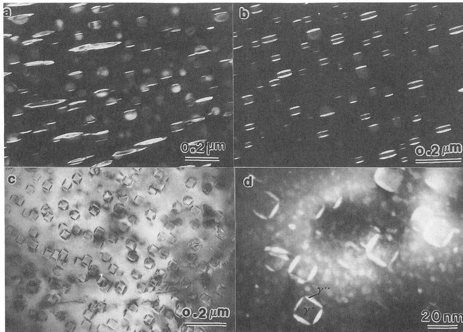
Fig.16 Associated precipitation and compact morphology of  $\gamma''$  and  $\gamma'$  in Alloy 13 (a-dark field) and Alloy 15 (b, d-dark field, c-bright field) after long time aging at 730°C for 200hrs
