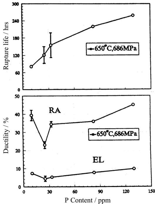
Fig.11 Effect of phosphorus on 650°C, 686MPa stress rupture life (a) and ductility (b) on IN718
