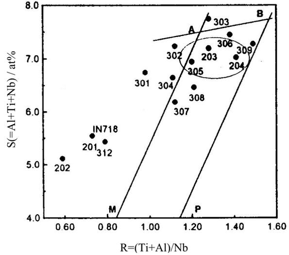
Fig.18 Chemical composition distribution of modified 718 alloys in S-R coordinate
