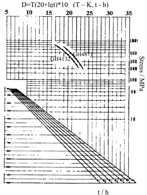
Fig.2 Stress rupture property comparison between GH4871 and GH4132 (A-286)
