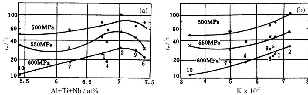
Fig.19 Dependence of 700°C creep fracture time on atomic sum of Al+Ti+Nb (a) and on coefficient K at 500, 550, 600MPa (b)
