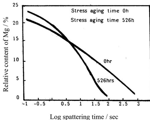
Fig.6 Grain boundary segregation behaviour of Mg in Mg-containing alloy (59ppm) 718M before and after stress aging at 650°C, 686MPa
