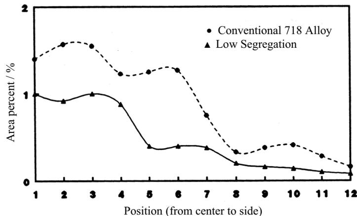
Fig.10 Distribution of blocky-Laves fraction in  $\phi$  406 Inconel 718 ingots
