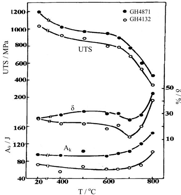
Fig.1 Tensile property comparison between GH4871 and GH4132 (A-286)
