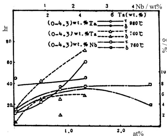
Fig.24 The influence of Ta and Nb in alloys on stress rupture properties at 760°C, 647MPa; 980°C, 200MPa
