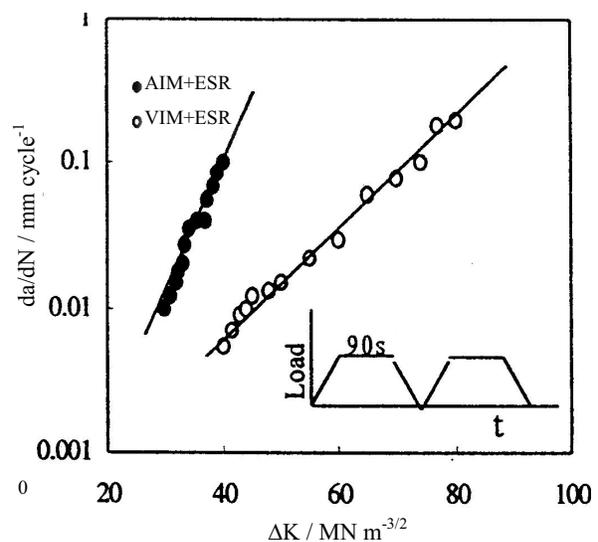
Fig.5 Crack growth rate behaviour of air melted (AIM+ESR) and vacuum melted (VIM+ESR) GH4871 alloys at 650°C and 90 sec dwelling time at maximum loading
