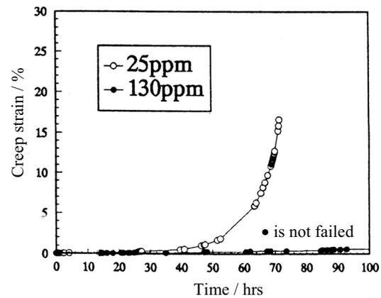
Fig.12 Effect of phosphorus on creep curves of IN718 at 650°C, 725MPa
