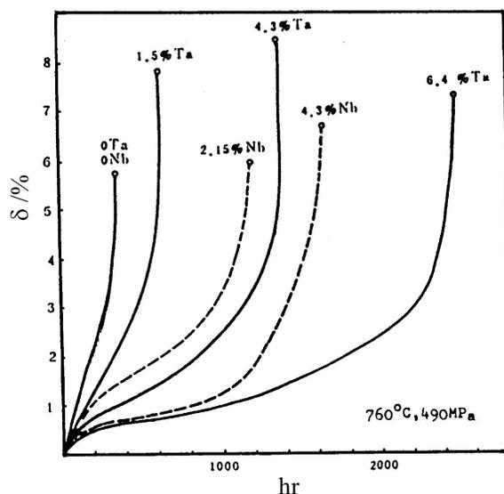
Fig.25 The creep curves of alloys with various contents of Ta and Nb
