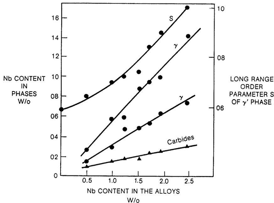
Figure 1: Partitioning of niobium to  $\gamma$ ,  $\gamma'$  and the carbides along with the long-range order parameter "S" of  $\gamma'$  in solid solution nickel-base alloys containing 0 to 2.5% niobium (1).
