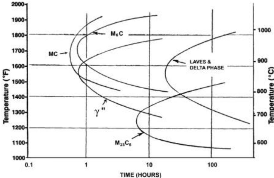
Figure 5: Suggested Time-Temperature-Transformation Diagram for alloy 625 (12).
