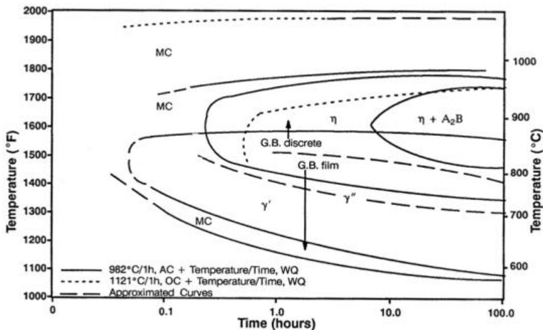
Figure 7: Approximate time-temperature-transformation diagram for alloy 706 (23).
