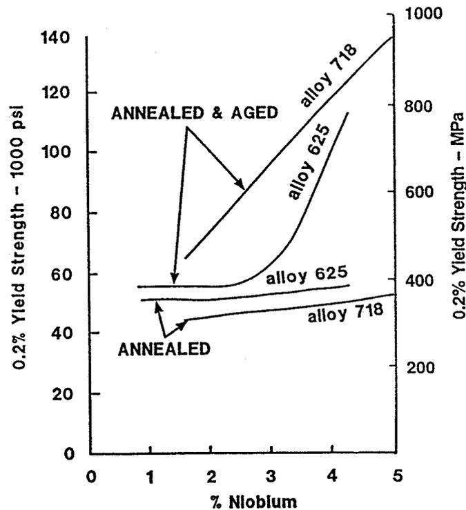
Figure 4: Effect of niobium additions on the 0.2% yield strength of the base compositions of alloys 625 and 718 (9).
