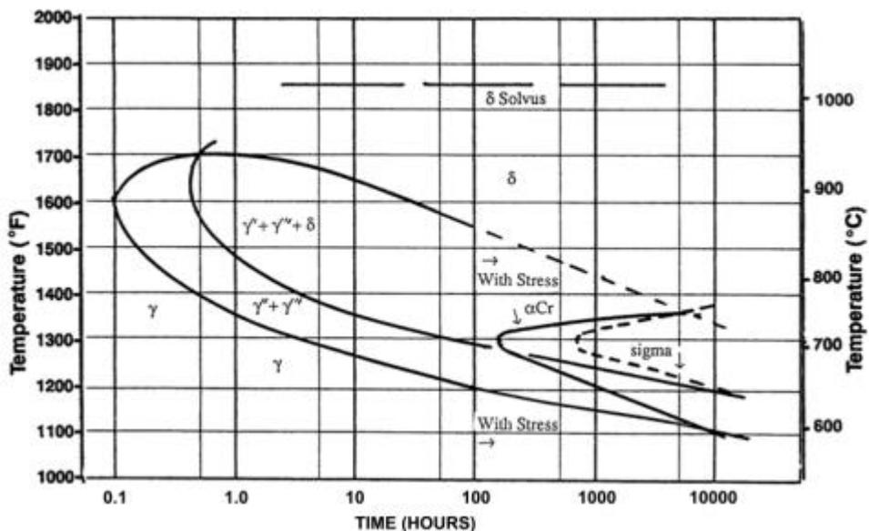
Figure 9: Time-Temperature-Transformation diagram for alloy 718 (45).
