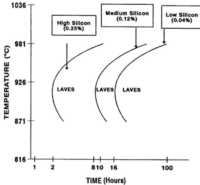
Figure 8: Time-Temperature-Transformation diagram showing the effect of silicon content on the formation of Laves phase in alloy 706 (34).
