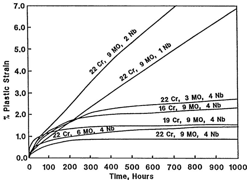
Figure 3: Creep Tests at 52 MPa/816°C for a range of niobium, molybdenum and chromium additions to nickel (9).
