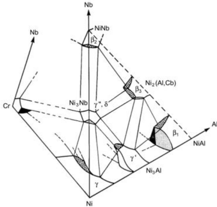
Figure 6: Sketch of the approximate relationships between  $\gamma$ ,  $\gamma'$ ,  $\gamma''$  and  $\delta$  in the nickel-aluminum-chromium-niobium system.
