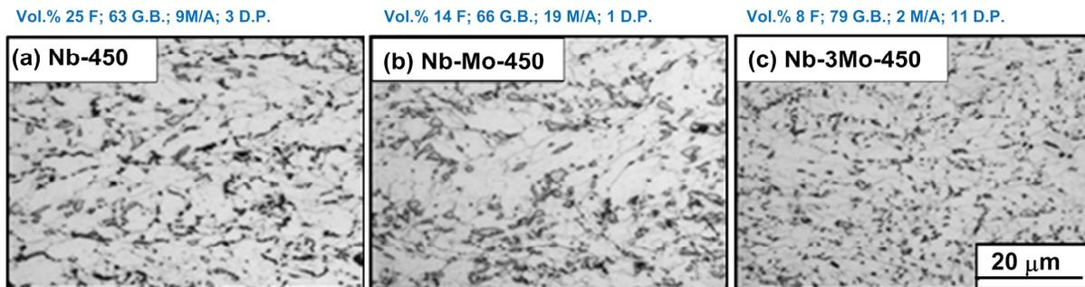
Figure 4. OM micrographs showing the microstructures of; (a) Nb-450, (b) Nb-Mo-450, (c) Nb-3Mo-450. Granular bainite (G.B.), allotropic ferrite (F), martensite/austenite constituents (M/A), and degenerate pearlite (D.P.).
