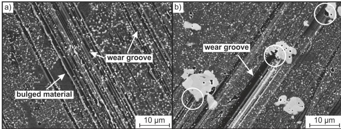
Figure 9. SEM images of worn surfaces of a) PSH1, b) MMC after scratch tests with flint 220. The wear grooves and bulged material at the edge of the grooves are obvious in PSH1. In the MMC, sections of the wear groove indicated by circles show where the abrasive particles were stopped or deflected.
