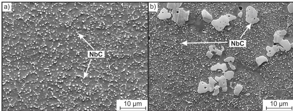
Figure 7. SEM images of the microstructure of; (a) PSH1 and (b) MMC [18] after HIP in the as-quenched condition ( $T_{\text{Aus}} = 1100\text{ }^{\circ}\text{C}$ ). The finely dispersed NbC that precipitated during diffusion alloying have a diameter in the range of 1–3  $\mu\text{m}$  and are thus even smaller than in the hardfacing alloy, Figure 3(b). The admixed NbC in the MMC are considerably larger (about 10  $\mu\text{m}$  in diameter). Their distribution is not totally homogeneous.
