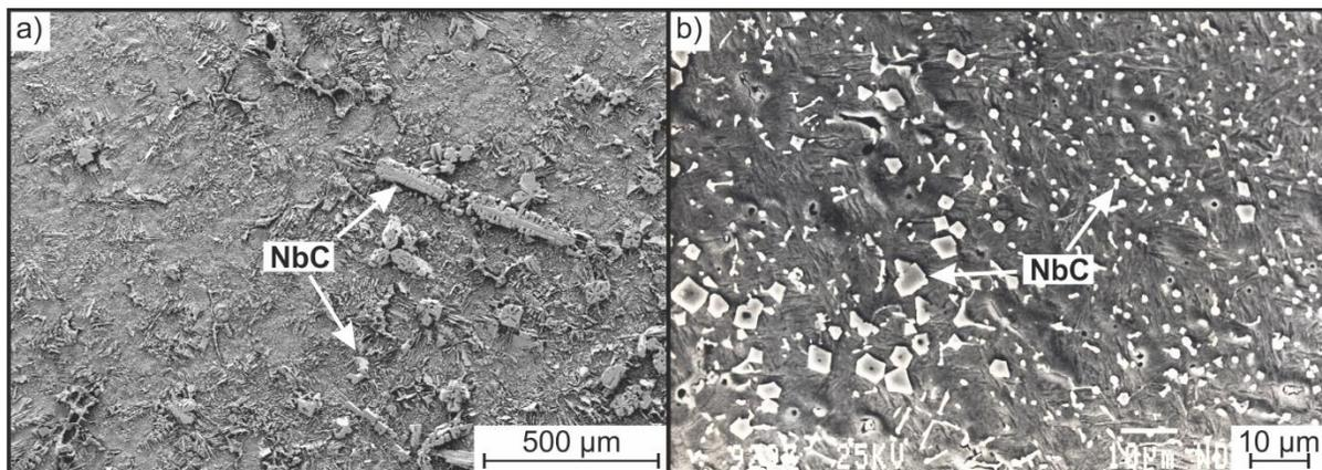
Figure 3. Different morphologies of NbC; (a) huge NbC in alloy G-X130NbCrMoW6-4-2-2 in the as-cast condition, (b) fine dispersion of NbC, comparable to a powder metallurgical microstructure, in hardfacing alloy X120NbCrMoV6-5-2-1.
