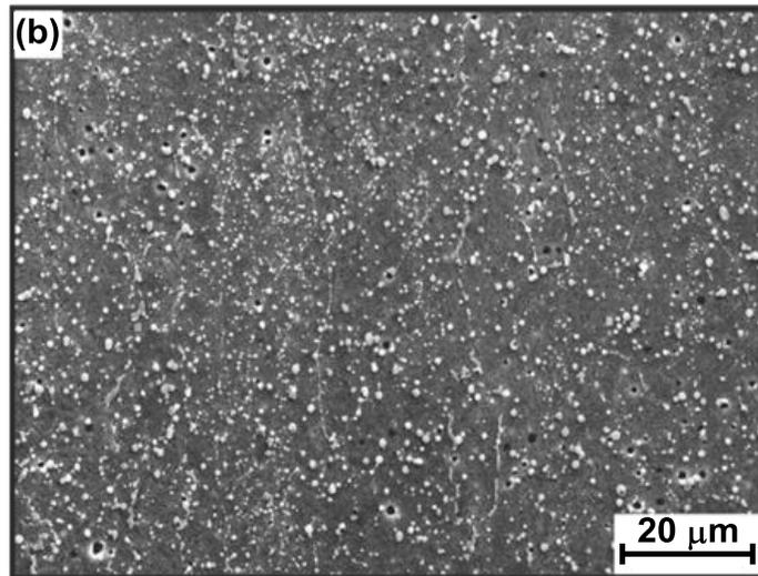
Figure 12. (a) Tempering curve of NBS (grey dashed line). Its hardness is in the range of that of PSH1 (solid line) and MMC (black dashed line) and well above 650 HV. (b) Microstructure of the new bearing steel. As intended, the content of NbC is reduced in comparison to PSH1 and MMC.
