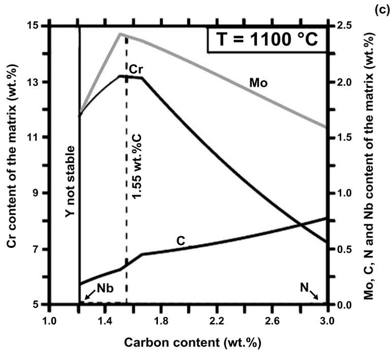
Figure 2. Different equilibrium properties at 1100 °C depending on the carbon content calculated with Thermo-Calc. The dashed line indicates a carbon content of interest for this study; (a) Phase content in vol.%, (b) Composition of the NbC, (c) Composition of the matrix. The x axis in (c) is scaled only from 1.0 to 3.0 wt.%C because the austenite is not stable below  $\approx 1.2$  wt.%, which is also shown in the diagram.
