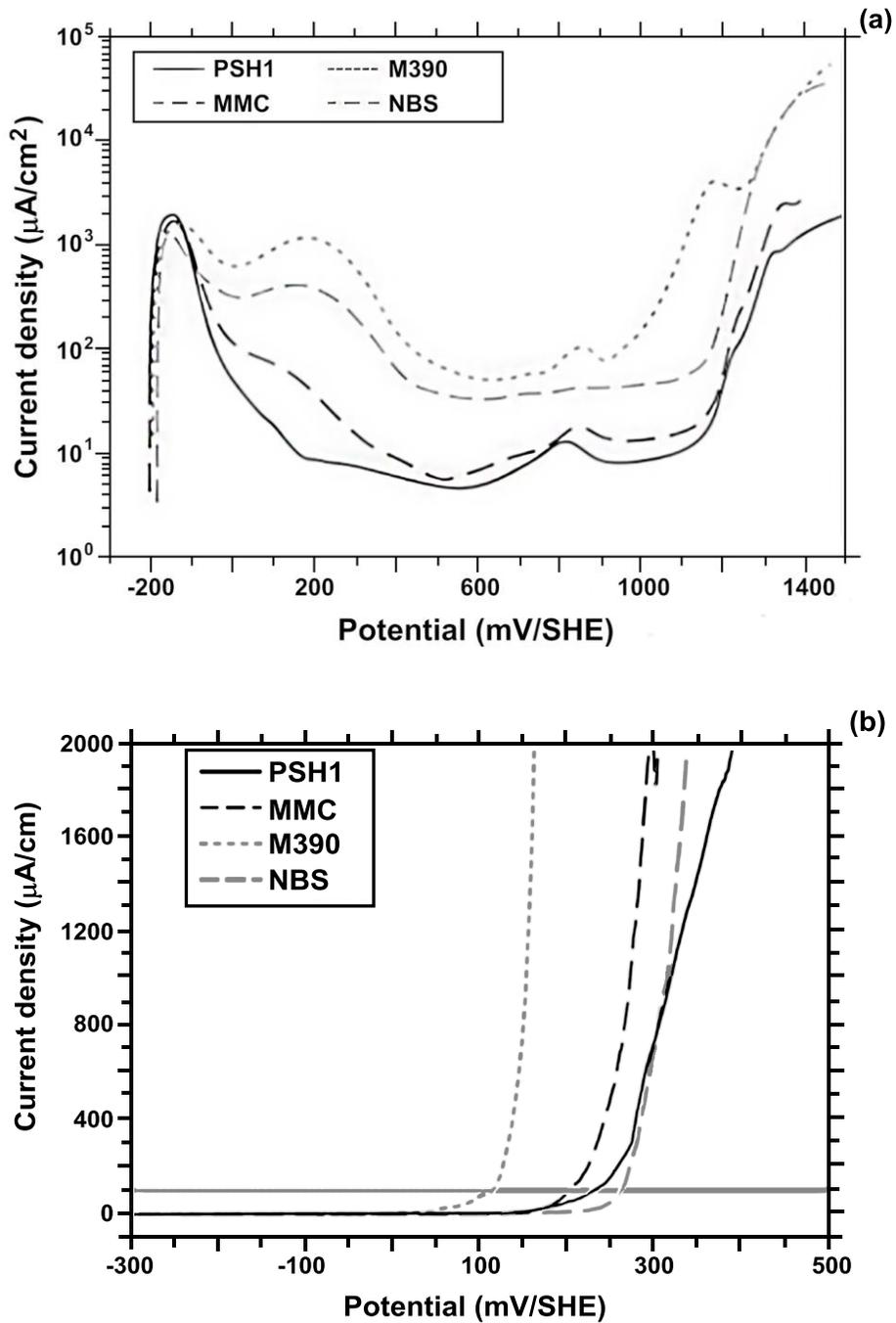
Figure 13. Representative potentiodynamic polarisation curves for NBS (grey dashed line) compared to the curves shown in Figure 11; (a) in H<sub>2</sub>SO<sub>4</sub> and (b) in NaCl. The NBS was tested in the as-quenched condition that is comparable to the other three steels. In H<sub>2</sub>SO<sub>4</sub>, the corrosion resistance of the NBS is higher than that of M390, but lower than that of PSH1 and MMC. In NaCl the NBS shows the highest corrosion resistance of all four alloys.
