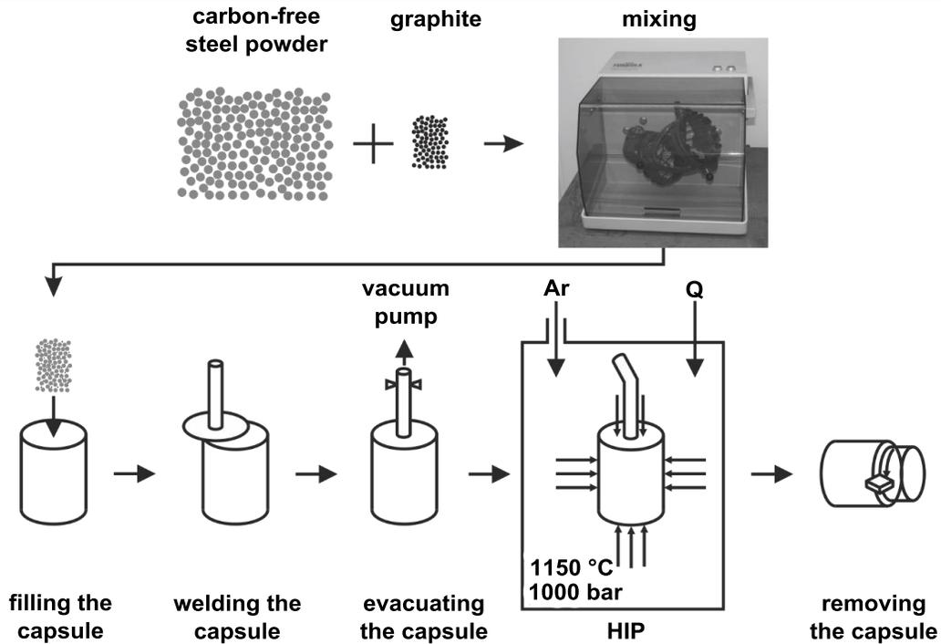
Figure 4. Schematic sequence of diffusion alloying including the HIP process, where Q indicates heat (according to [31]).
