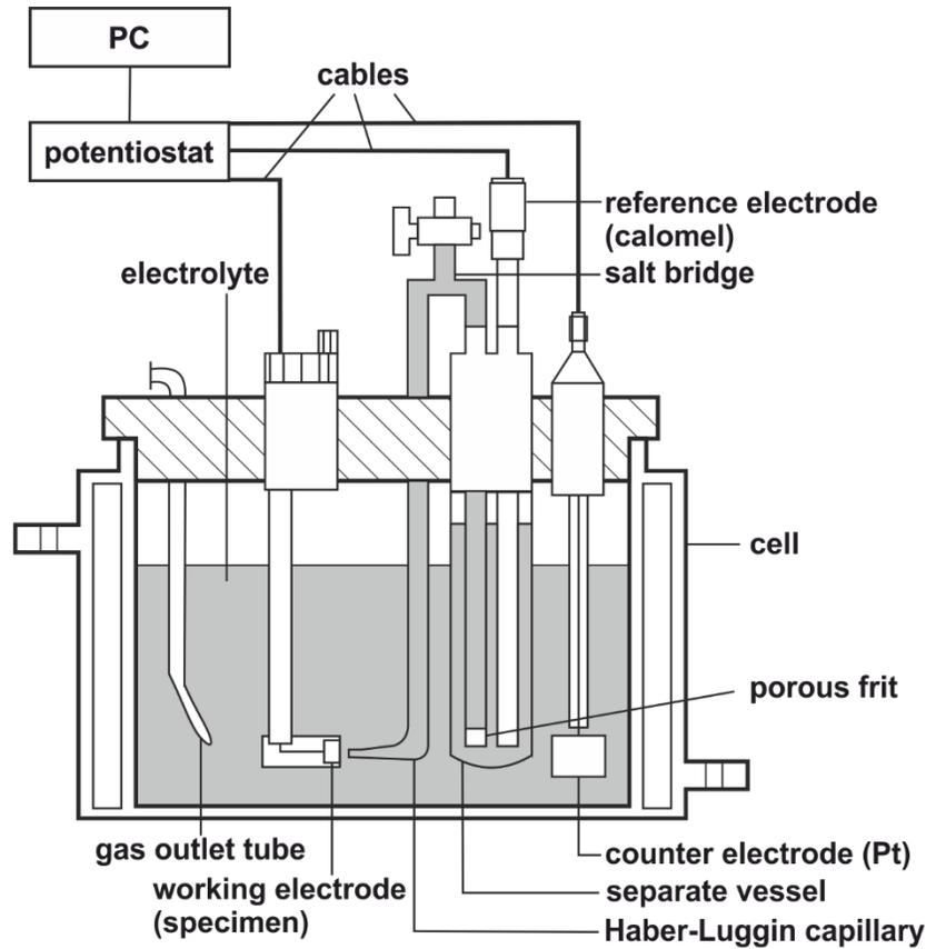
Figure 6. Schematic illustration of the corrosion test setup used to measure potentiodynamic polarisation curves. The electrolyte – either  $\text{H}_2\text{SO}_4$  or  $\text{NaCl}$  – is coloured in grey.
