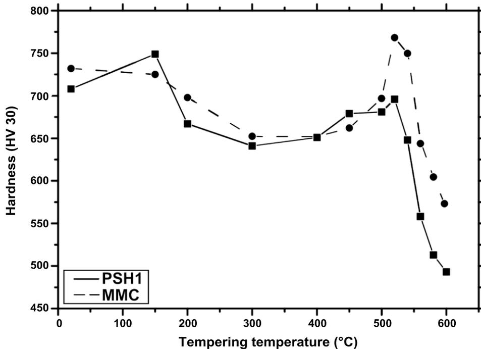
Figure 8. Tempering curves for the two investigated alloys PSH1 and MMC in the range from room temperature to 600 °C for hardening from 1100 °C. The as-quenched hardness of both steels is comparable. The SHM is reached for tempering at 520 °C with MMC and achieves a higher hardness than PSH1.
