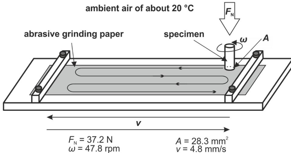
Figure 5. Schematic illustration of the pin-on-grinding paper test. The grinding paper is flint ( $\text{SiO}_2$ ) of mesh size 220 and 80 or corundum ( $\text{Al}_2\text{O}_3$ ) with a mesh size of 220. The area  $A$  of the specimen is given in the caption as well as the normal force  $F_N$  applied to the specimen, the rotational speed  $\omega$  of the specimen and the feed rate  $v$  of the grinding paper (table).
