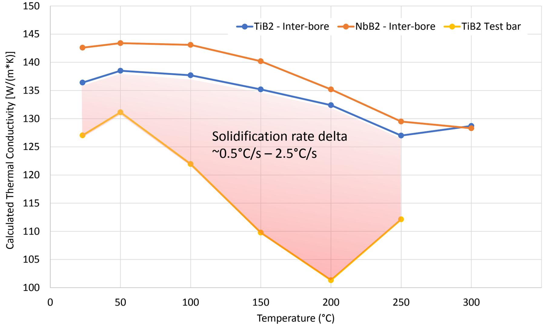
Thermal conductivity was calculated using the thermal diffusivity, density, and heat capacity of the material.
