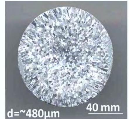
Extensive research showed Niobium to significantly reduce the grain size in AlSi alloys over industry established Titanium grain refiner.
