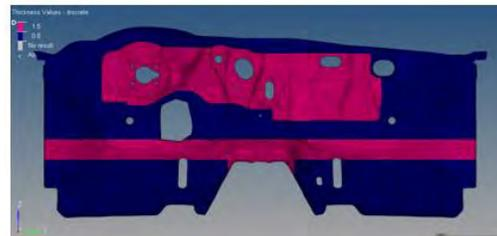
Dashboard panels exhibit low levels of mobility. MaX solution satisfies guidelines and shows only a minor difference in performance over the baseline. Note that the increases observed are likely to be at only a few points where refined geometric improvements may help.
