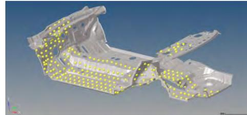
Panel mobility is assessed by applying a unit load normal to the panel surface and calculating the resulting velocity across all panels
