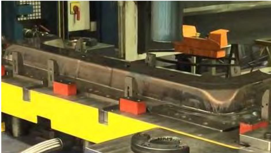
Final parts obtained by using standard procedures. Good results in terms of hole expansion.
