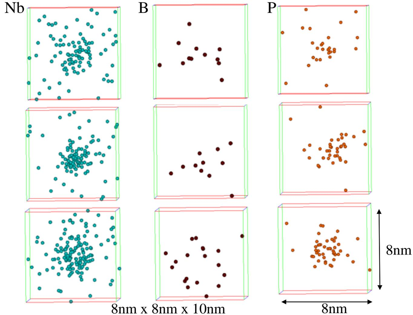
Most of the excess Nb atoms are observed within a small circle 2~3 nm in diameter.
