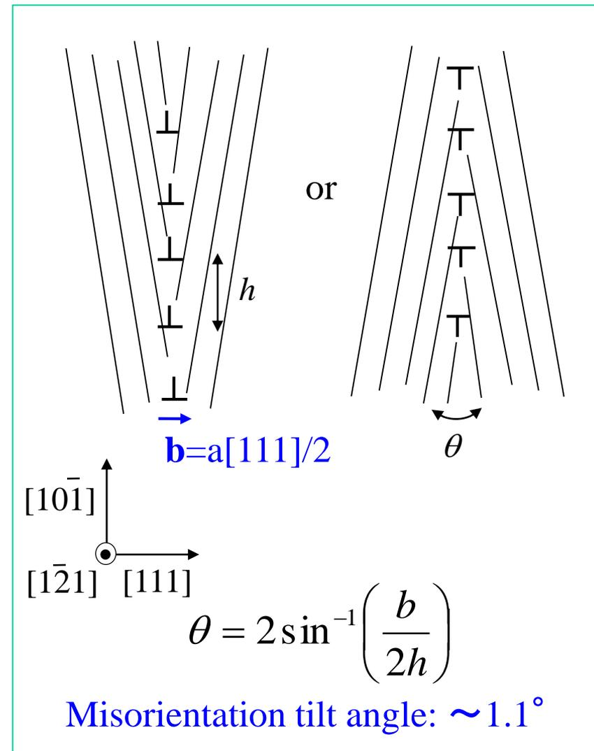
Low-angle tilt grain boundary on (111), composed of pure edge dislocations
