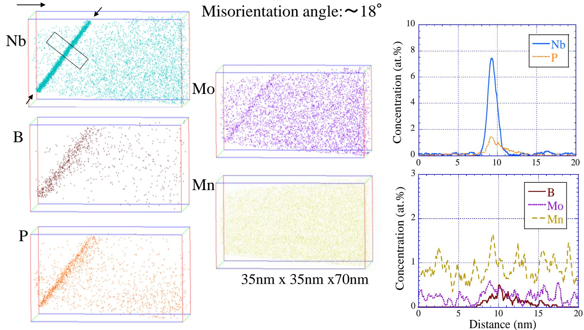
Planar like heavy segregation of Nb is observed at the grain boundary.
