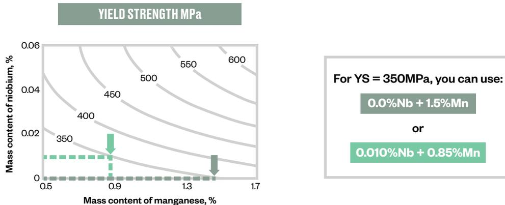
Therefore, the application of the lean alloy design using niobium to reduce the amount of manganese required, enables the mechanical properties to remain the same. Furthermore, up to 355MPa, Thermomechanical Controlled Processing (TMCP) during rolling is also not required to meet the required mechanical properties.
